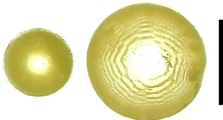
Fig. 1. The two-dimensional precipitation patterns of lead iodine in agarose gel at 22.0 \pm 1.0 °C: R_0 = 4 mm (left) and R_0 = 7 mm (right). The scale bar is 1 cm.
