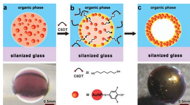
Fig. 1 Preparation and appearance of NP-armoured droplets. (a) Droplet containing basic solution of AuNPs functionalized with DFMP ligands is placed onto silanized glass immersed in an organic solvent. The optical image in the bottom row shows that this droplet appears dark red due to the SPR of the free NPs. (b) When 10\ \mu\text{M} HS-(CH 2 ) 6 -SH, insoluble in water, is added to the organic phase, it crosslinks the NPs at the interface. (c) As more and more NPs reach the interface and are cross-linked therein, the nanoparticulate armour develops a characteristic metallic gloss.
