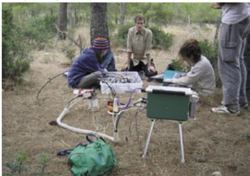
Did you know that the soil was respiring? With this 'soil chamber' we are measuring how much CO 2 Pianosa's ground is emitting
