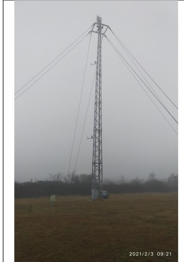
Figure 1: 30-m meteorological tower for temperature and wind profile measurements along with eddy covariance measurements done at the top (30 m) using Gill sonic Windmaster 3D anemometer.
